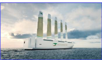
The wPCC uses four sails or wings mounted on its roof to catch the wind and propel it forward. It's not as fast as fossil fuel cargo ships, but it's substantially greener. The transatlantic ship capable of carrying up to 7,000 vehicles and reducing emissions for the crossing by 90%. And it's powered directly by wind.
